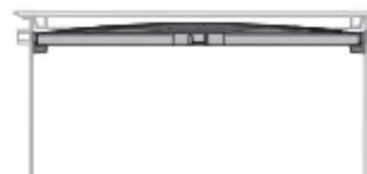
Orenco's Tank Shield locks securely into mounting brackets without the need for additional bolts or screws.
